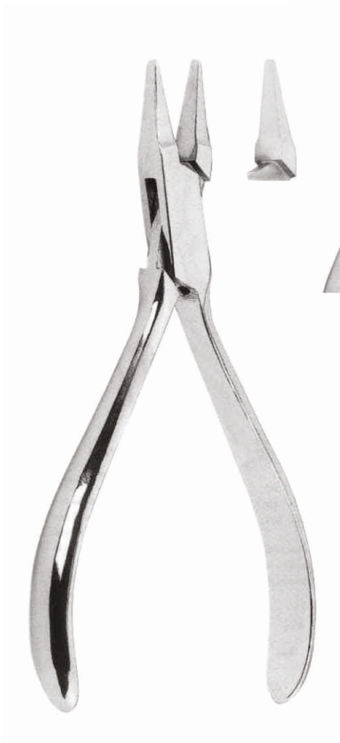
SF-04-40984 Flat nose pliers with smooth beaks for bending wires up to 0,7 mm. (.028").
