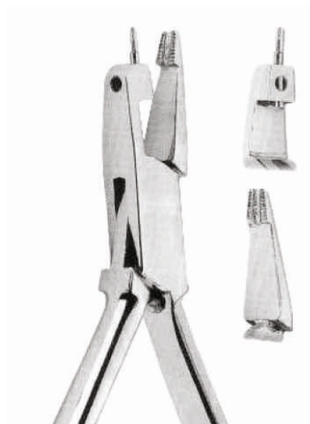
SF-04-40995 De La Rosa De La Rosa arch forming pliers. Designed to form and contour arch wires on round or rectangular wire. The beak has grooves of 0,4 mm (.016"), 0,46 mm (.018") and 0,56 mm (.022").
